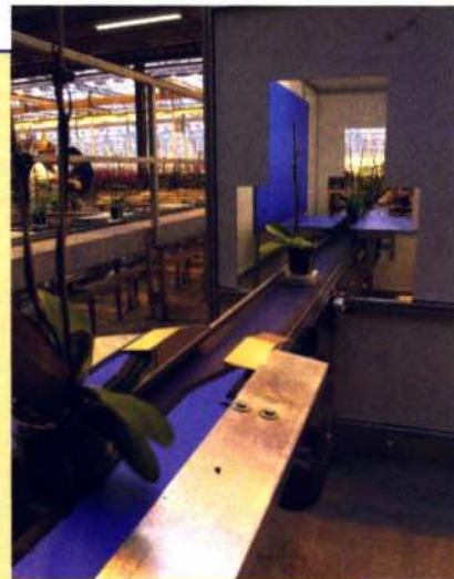
This vision system takes 360-degree pictures of plants and grades them according to criteria that is input into the program. (Photo: Logiqs Agro)
