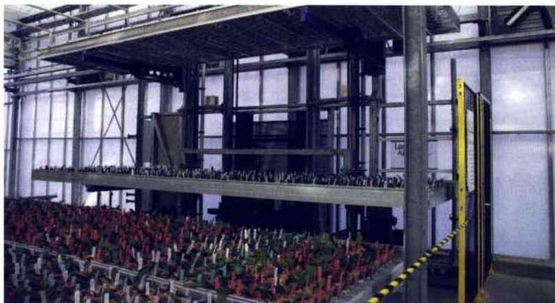
The table-moving robot literally lifts tables off the ground as it moves them to different production areas.
